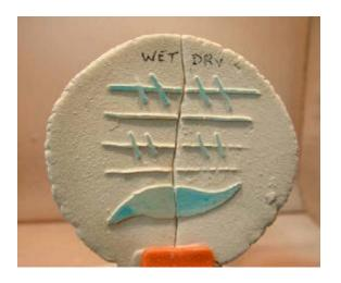
Surprise, surprise! It doesn't seem to make any difference. Given the choice, I'd choose the leather-hard stage, since it's less likely that the pot would be stressed when the freshly wet outer surface swells and strains against the still-dry interior.
